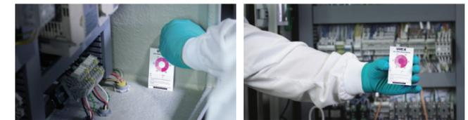
11. If the strip indicates UV-C rays lower than 75 mJ/cm<sup>2</sup>, ensure the unit is receiving power and the bulb or fuse is not burnt out. If a new bulb is needed, follow the directions in step 13.
