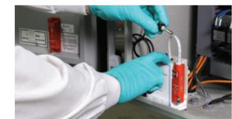
12. Record the date of bulb installation on the included label. Replace the bulb every 6 months.
