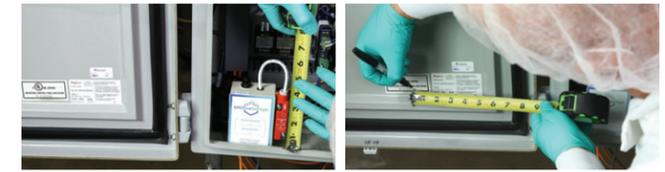
9. Remove the film from the magnet mounting tape and position on the door, applying gentle pressure for 30 seconds.
