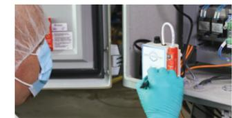
13. To replace the bulb, remove the old bulb by twisting it a quarter turn counterclockwise. Then, insert each end of the new bulb into the socket and twist a quarter turn clockwise.
